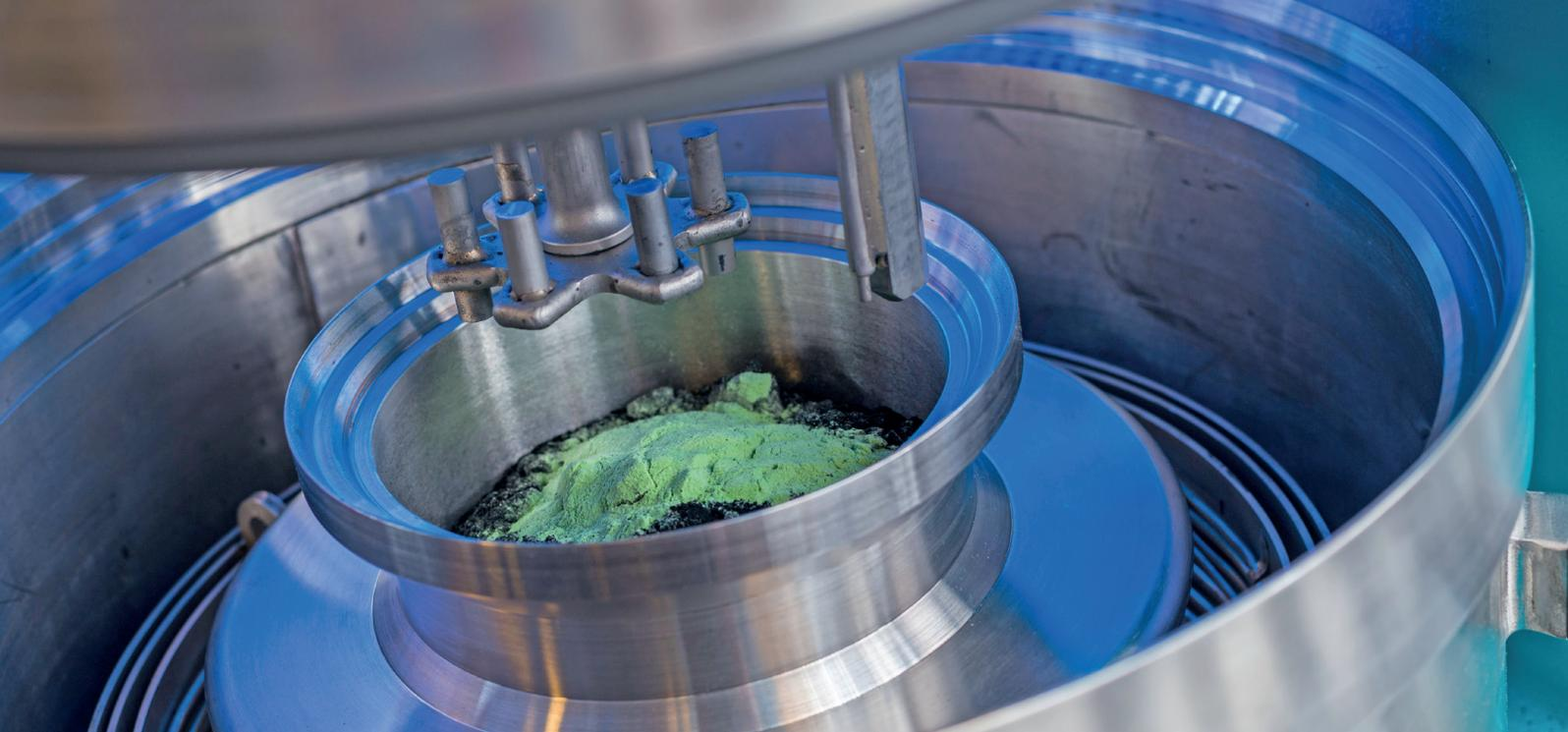
Vaku-Intensivmischer. ©Fraunhofer IFAM
