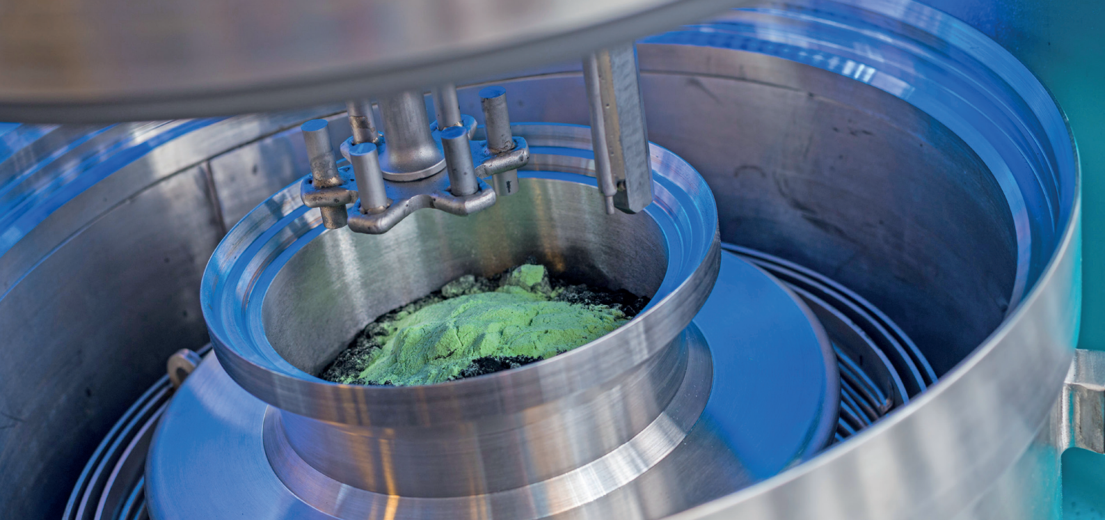
Vacuum intensive mixer. ©Fraunhofer IFAM
