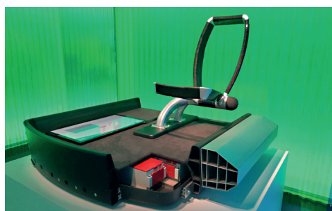
Exploded view of the SafeBat battery design with load-depen- dent heating of cell and module. ©Fraunhofer IWU
