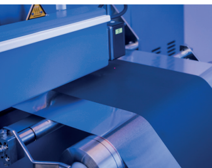
Continuous electrode manufacturing (©Fraunhofer IFAM).
